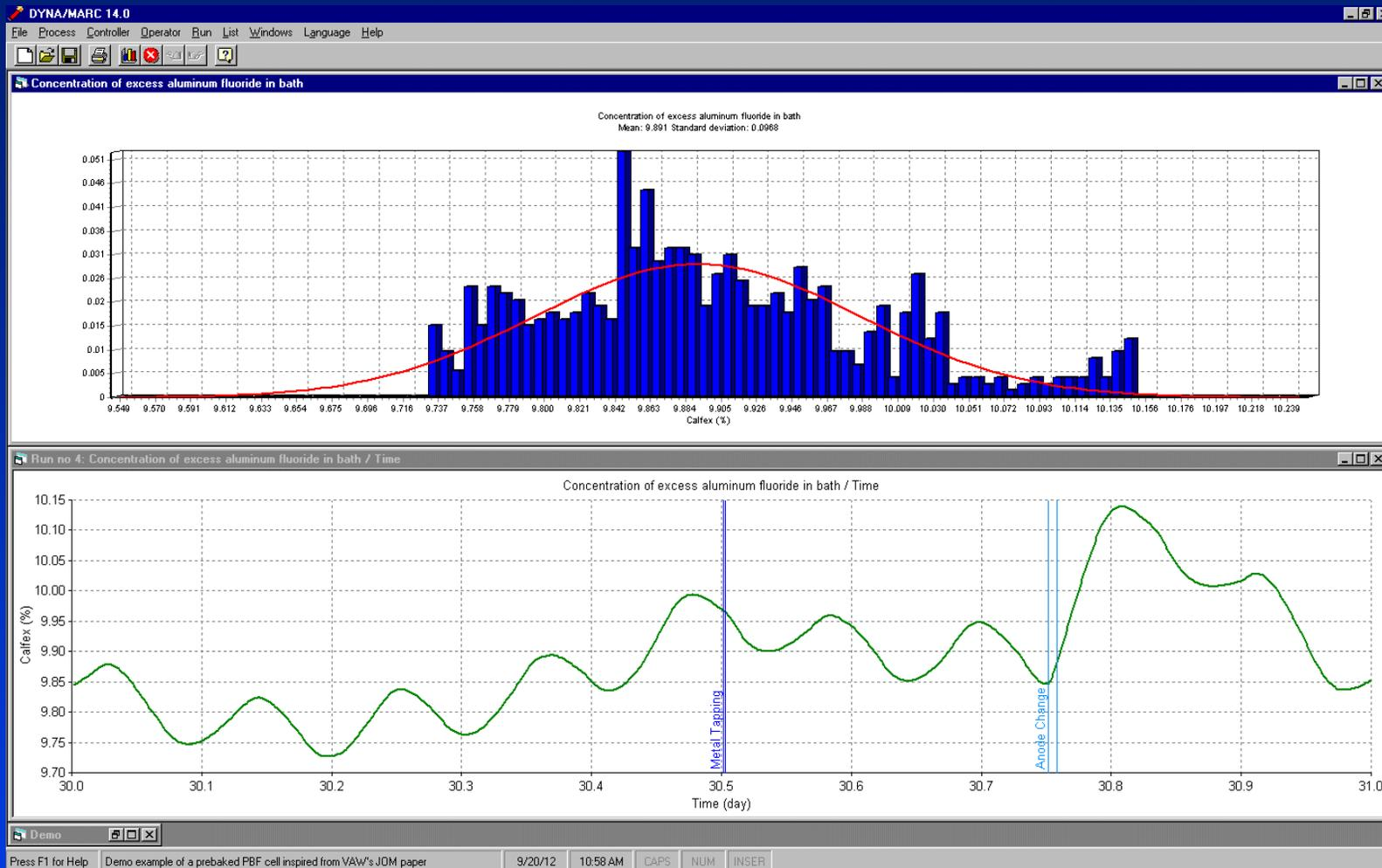
In addition of the irregular  $\text{AlF}_3$  addition, the excess  $\text{AlF}_3$  concentration variation is influenced by thermal events affecting the  $\text{AlF}_3$  evolution like the bath temperature but more importantly by the ledge thickness variation. Figure above shows the daily variation of the concentration of  $\text{AlF}_3$  in the bath in absence of control and any  $\text{AlF}_3$  mass imbalance. The standard deviation on the average value is about 0.1%.
