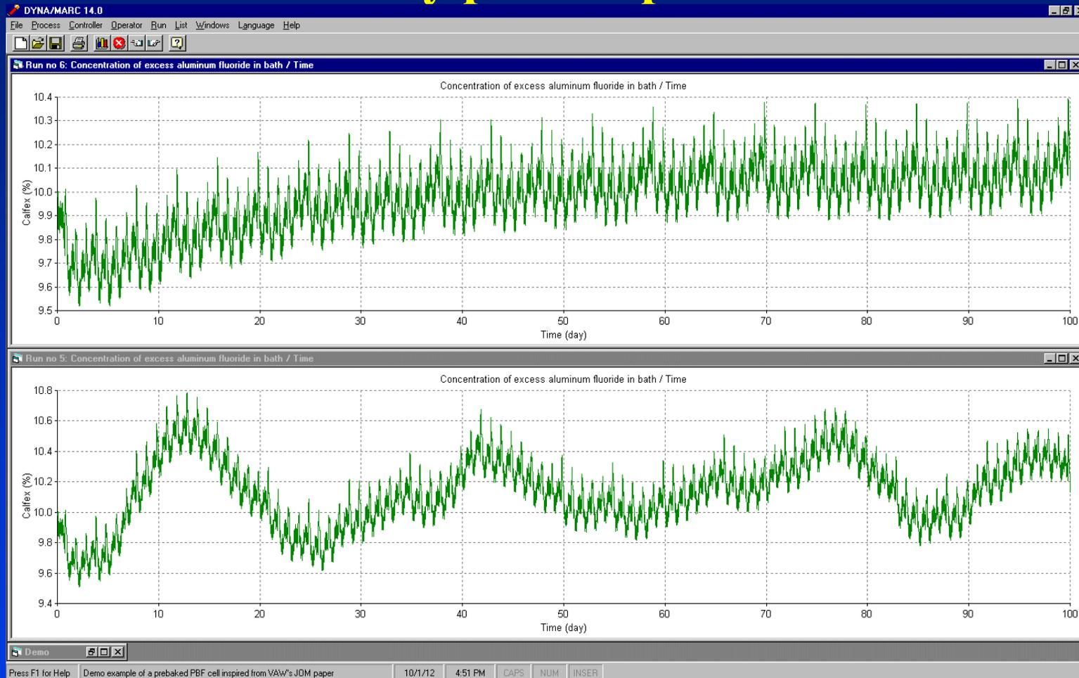
Simulation of the process without perturbation; top without control, bottom with feedback control, 10% target concentration: XRD results, once per day, 1 day delay, 0.5 kg/hr% proportional band and -0.1 kg/hr°C proportional band for temperature.
