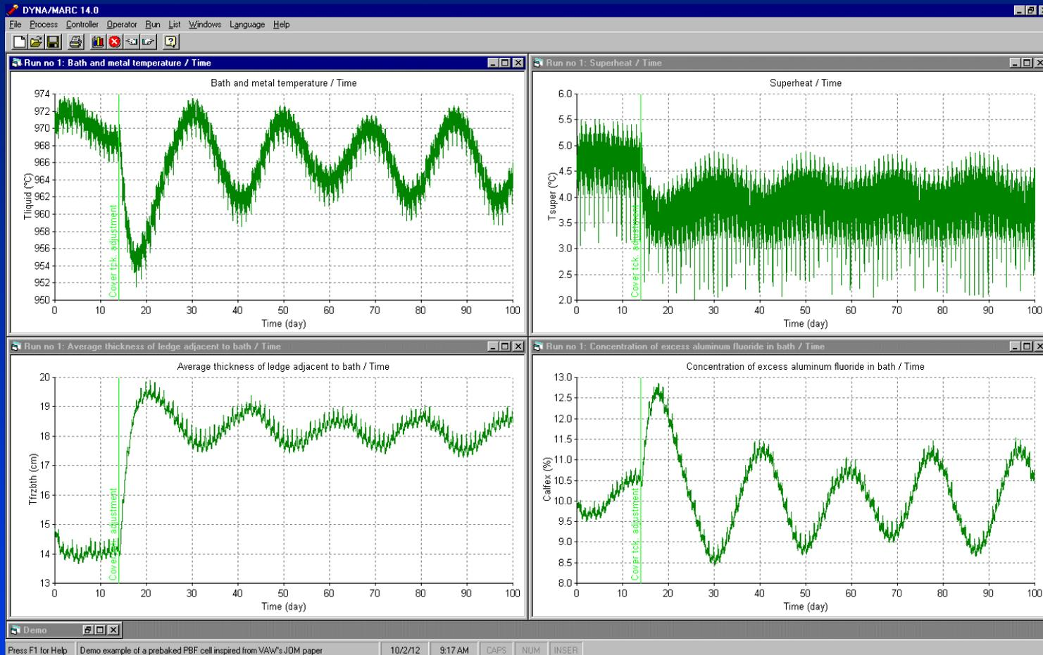
Figure above presents the results obtained using the standard control described above. After the change of superheat, the 970 °C temperature target is no longer compatible with the 10% excess  $\text{AlF}_3$  target, this combined with the 1 day offset between the  $\text{AlF}_3$  feedback and the temperature feedback generates a cyclic response characteristic of somewhat unstable feedback control.
