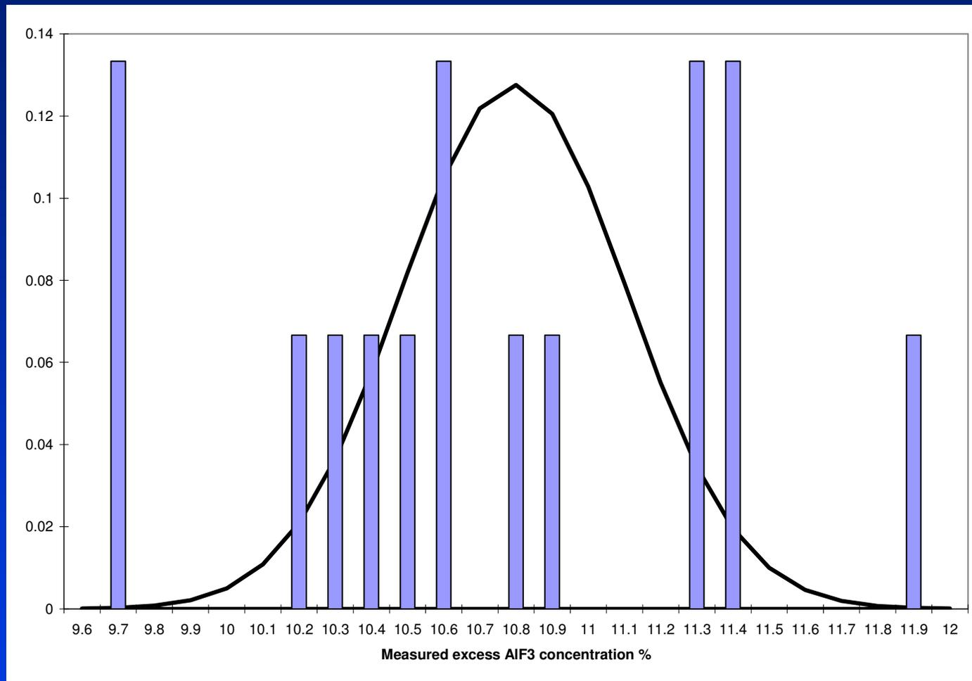
Figure above highlights the relative variability or lack of strict repetitiveness of the measurements which in turn highlight the lack of homogeneity of the bath. The standard deviation of that bath sampling noise has been evaluated to be around 0.5 % which is 5 times greater than the process noise generated by daily events (ref: ICSOBA 2012).
