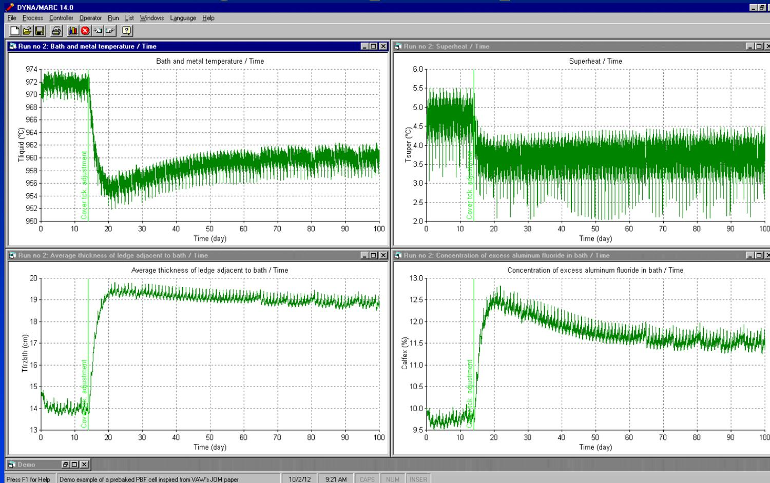
As we can see in figure above, as a natural response, the cell must reduce its cathode heat loss of the same amount by reducing its superheat by about 1 °C and increasing its ledge thickness by about 5 cm. As a result, of this extra ledge formation, the excess  $\text{AlF}_3$  increase by about 2% and remains close to 12% if the direct  $\text{AlF}_3$  additions remain unchanged.
